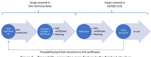
Figure 6 – Traceability connecting manufacture to the finished structure
